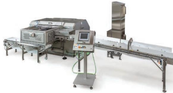
Danfotech bacon presses utilize a 3-dimensional press chamber to press bacon, Philly steak, roast beef and other products to increase slicing yield and efficiencies. Danfotech's technology does not use a conventional hydraulic press in the system. This results in water savings because water is not needed to cool the conventional hydraulic operated press.
